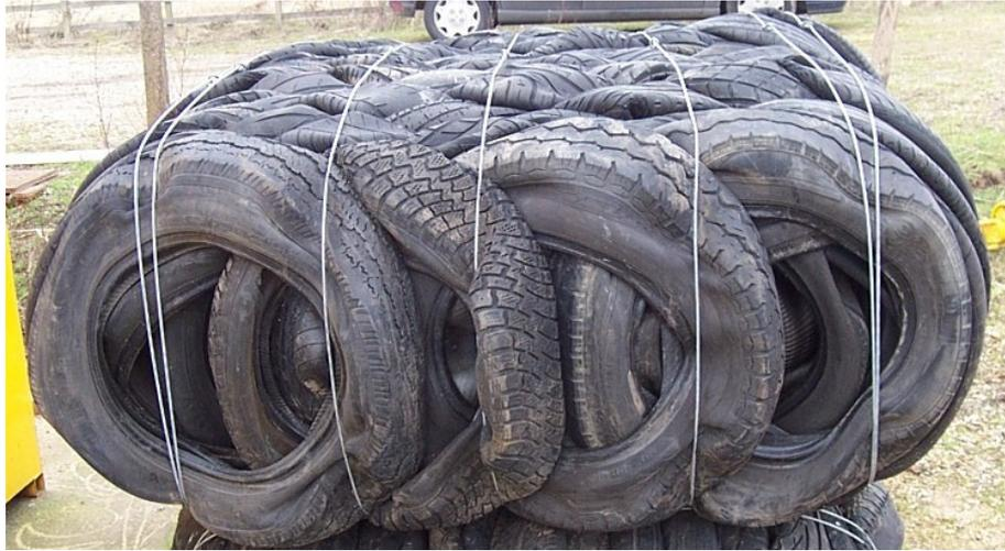
Figure 3. Tyre Bale (courtesy of HR Wallingford)
